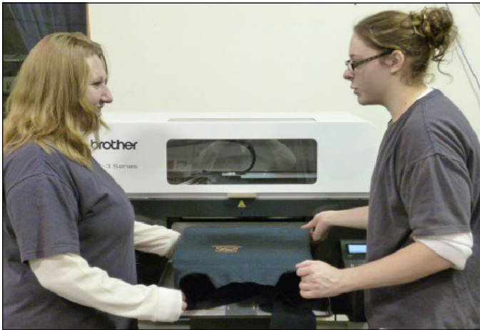
Offenders digitally print a multi-colored logo on a dark-colored shirt, a capability of the new Brother GT-381 garment printer.
