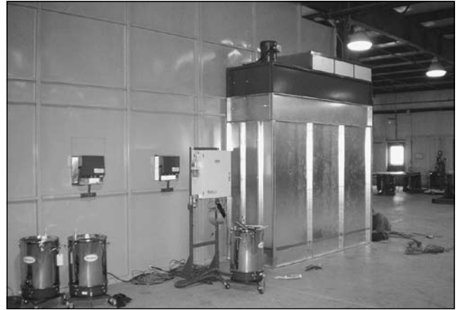
Outside view of collector and gun control system.
