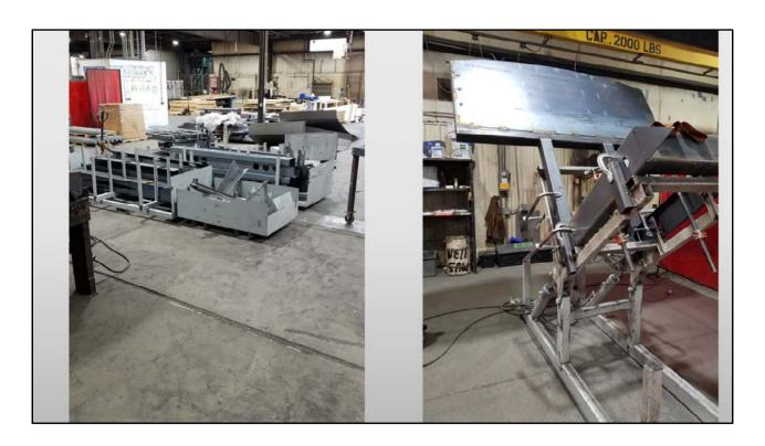
Typically the parts arrive in precut kits and with the associated drawings and jigs to hold everything in place, the welder then fabricates the part. They are palletized and prepped for pick up by Scranton Mfg.
